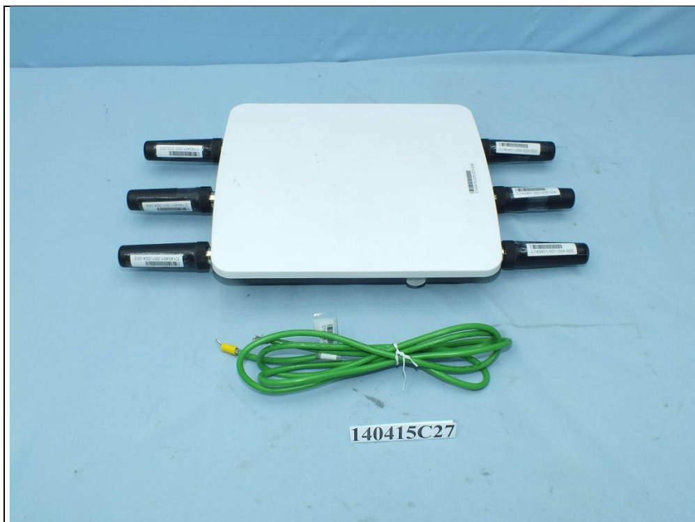
EUT with antenna 5 (Model: BMHODB2458IP)
