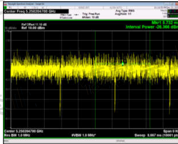
Tx. Spurious NVNT ax80 26@36 5210MHz Ant1 @ 5250MHz-5251MHz Final
