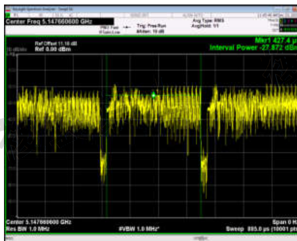
Tx. Spurious NVNT ax40 484@65 5190MHz Ant1 @ 5141.6MHz-5150MHz Final
