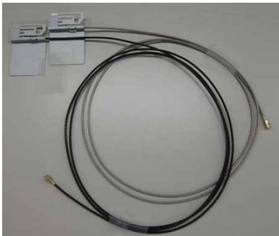
Antenna 4_ CP492500 (TX1) & CP492510 (TX2 or RX2) / NISSEI , 2010/12/01
