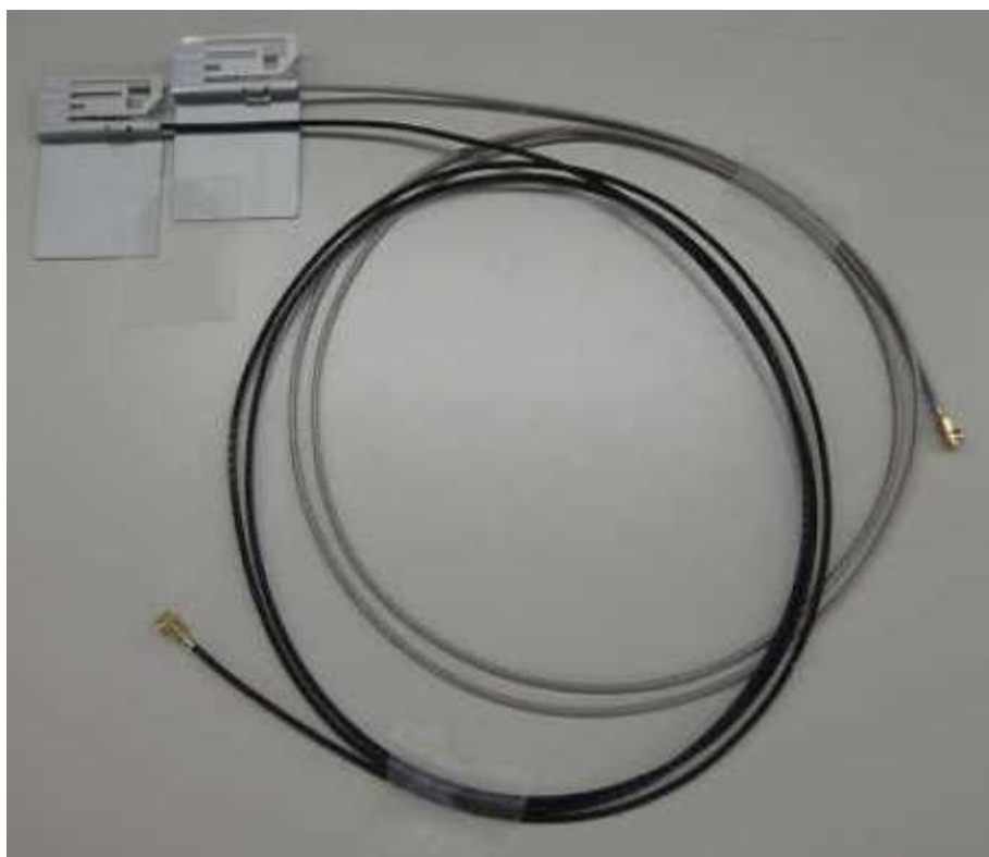
Antenna 8_ CP492501 (TX1) & CP492413 (TX2 or RX2) / NISSEI , 2010/12/01
