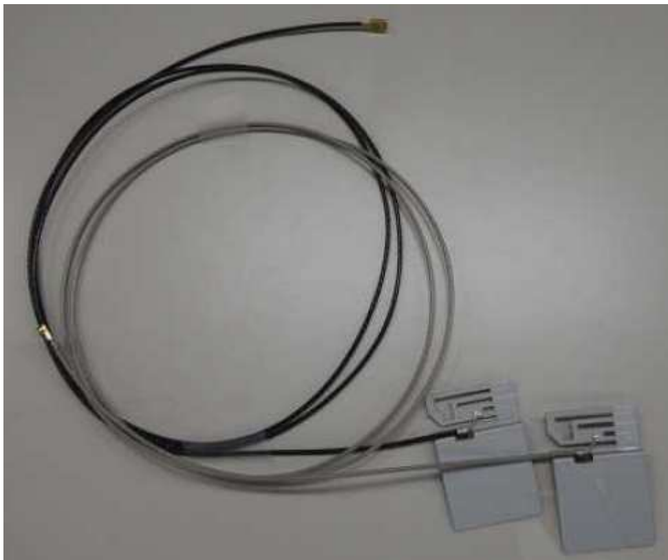
Antenna 2_ CP492498 (TX1) & CP492508 (TX2 or RX2) / NISSEI , 2010/12/01
