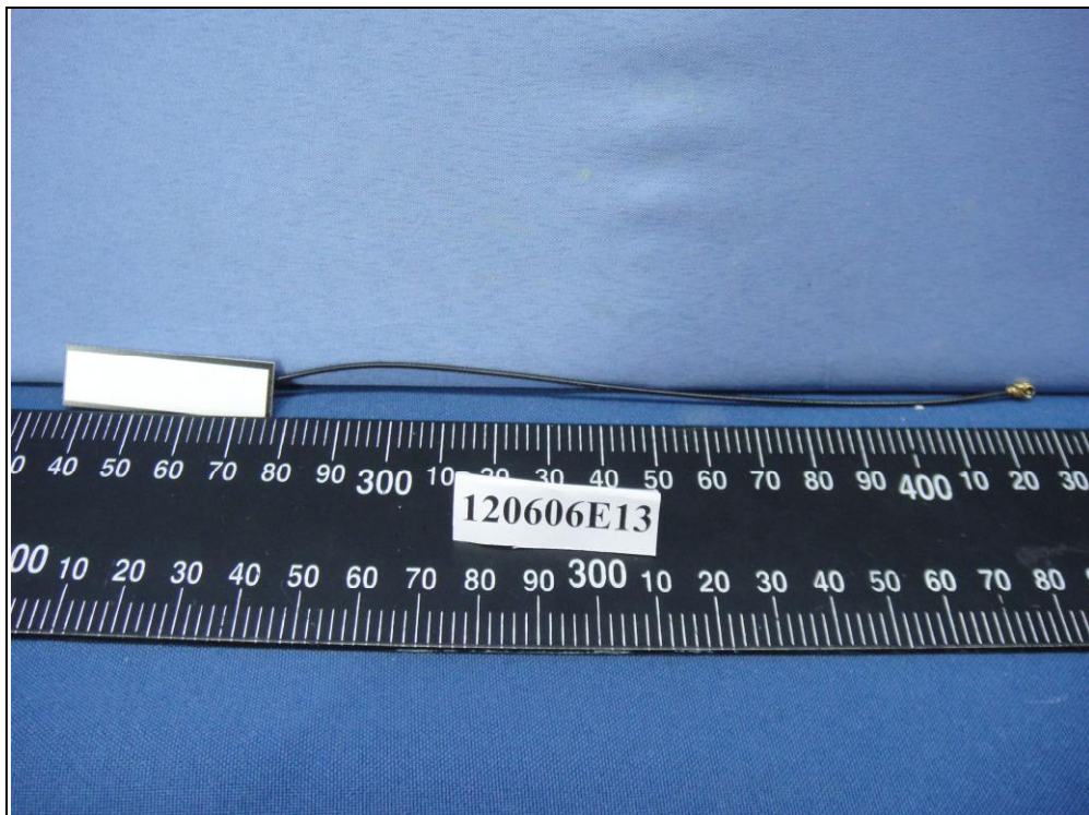
Antenna set 2 PCB Antenna (Brand name: ARISTOTLE ENTERPRISES, Model No.: RFA-02-P05-70B-150)
