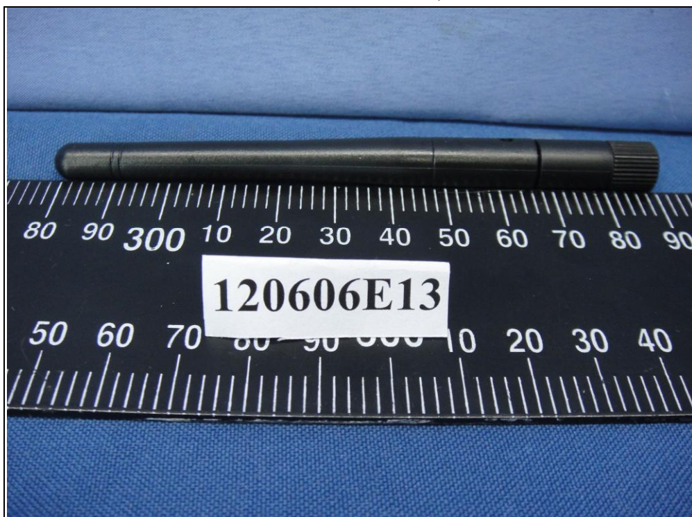
Antenna set 4 Dipole Antenna (Brand name: ARISTOTLE ENTERPRISES, Model No.: RFA-02-C2M2-M10-N)
