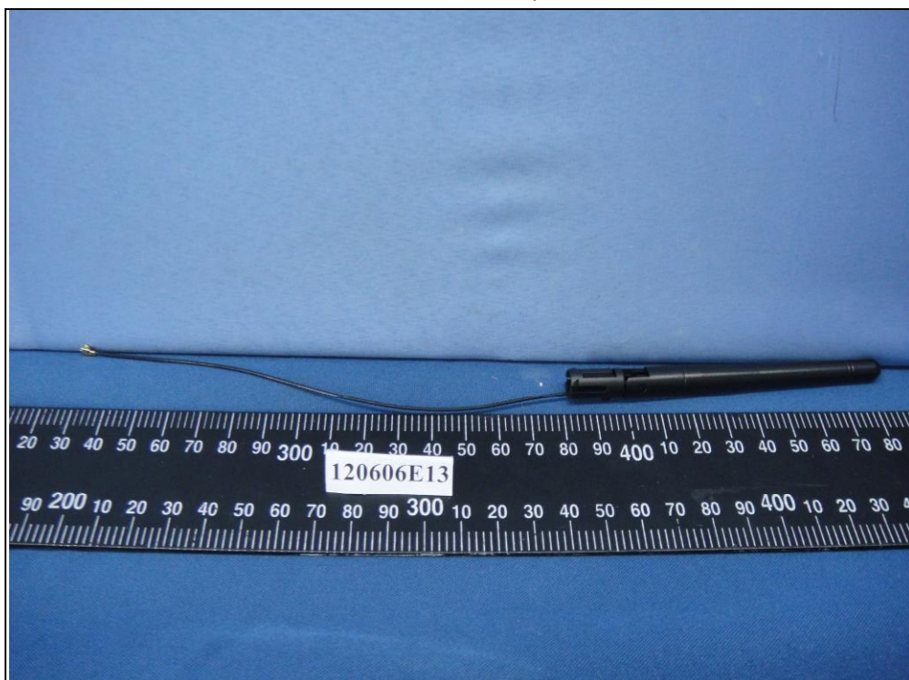
Antenna set 3 Dipole Antenna (Brand name: ARISTOTLE ENTERPRISES, Model No.: RFA-02-C2H1)
