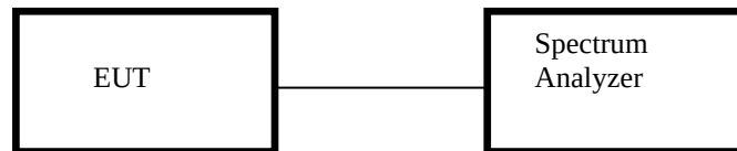
Figure 3. Frequency Error Test Configuration
