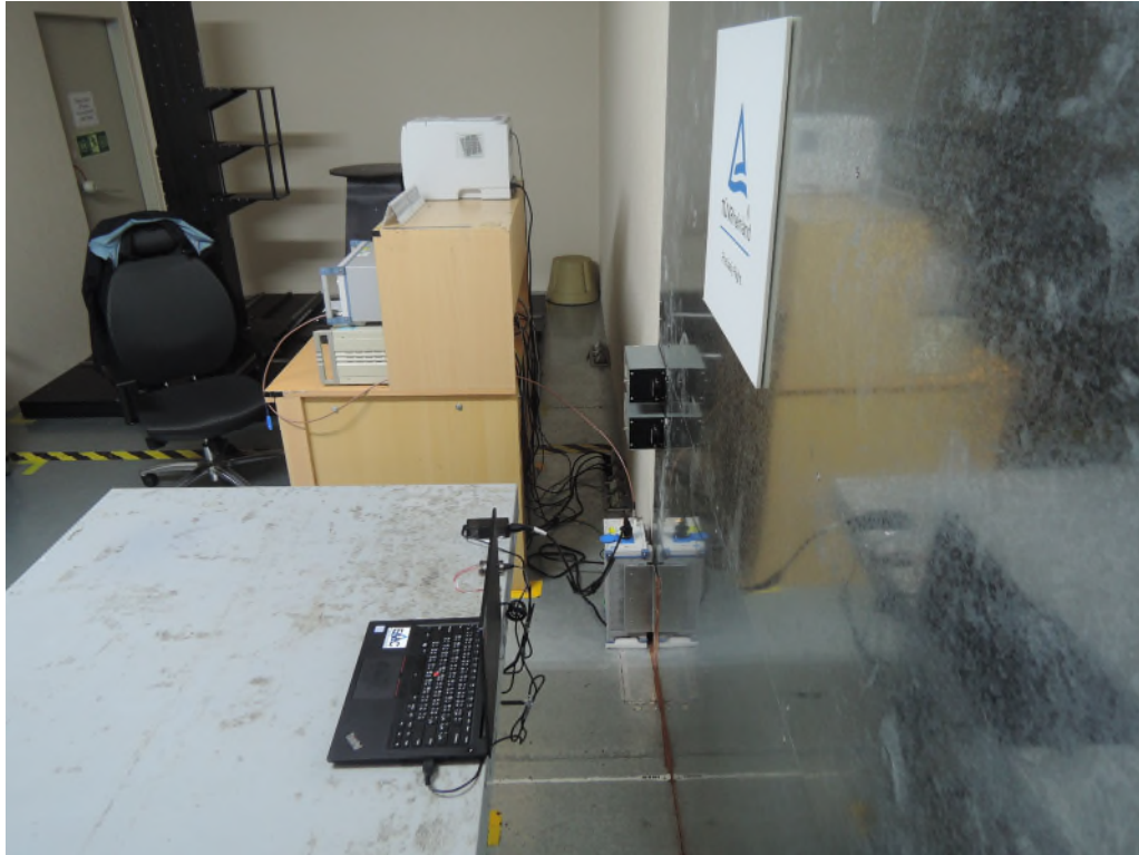
Photograph 5: Set-up for for Mains Conducted testing Back
