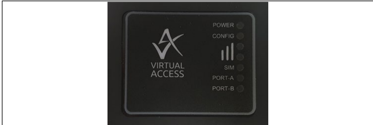
Figure 3: Exampe of a GW1150 top label showing LEDs (models may vary)
