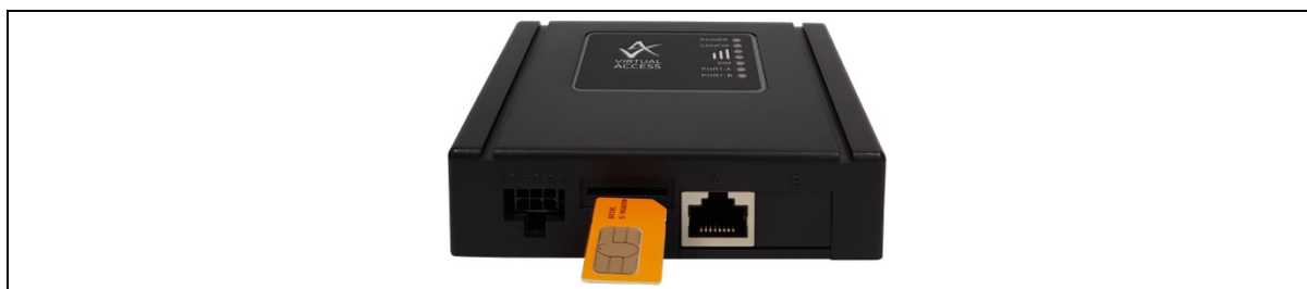
Figure 2: Inserting SIM card into SIM slot
