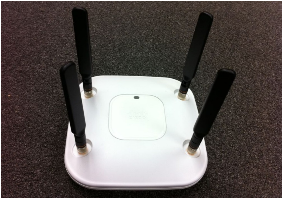
3602E with External Antennas Installed
