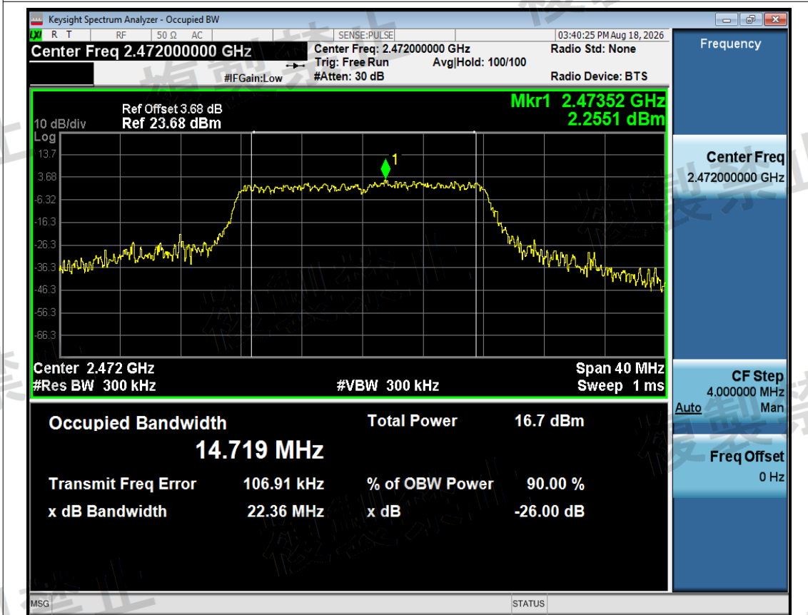
Spreading Bandwidth NVNT g 2472MHz Ant1
