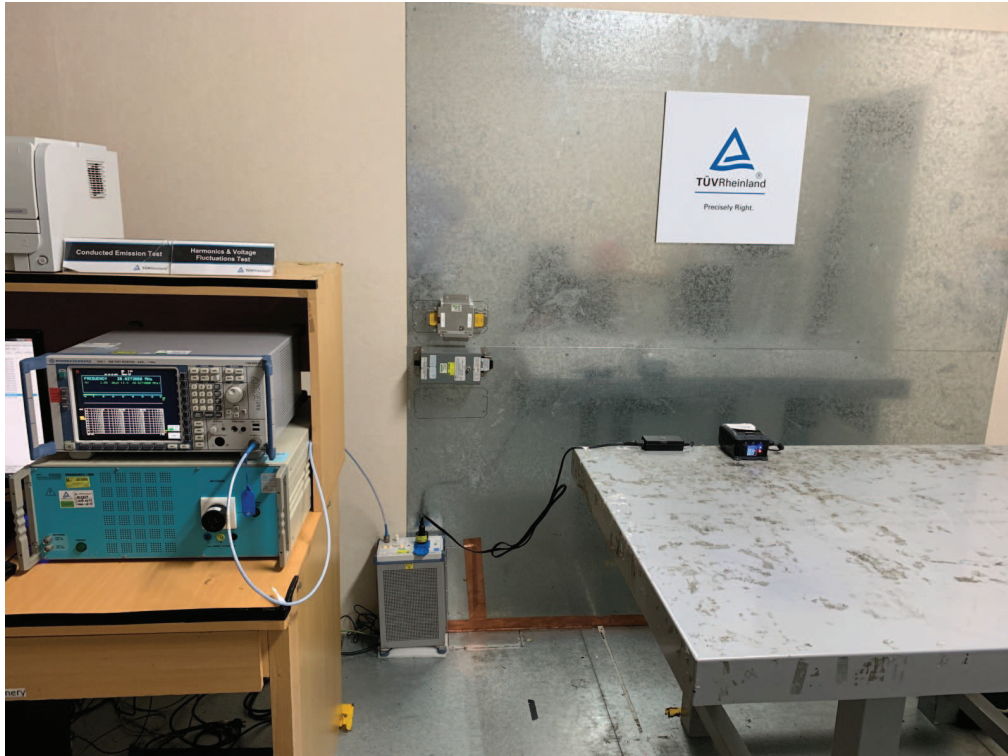
Photograph 7: Set-up for Mains Conducted testing (Front View)
