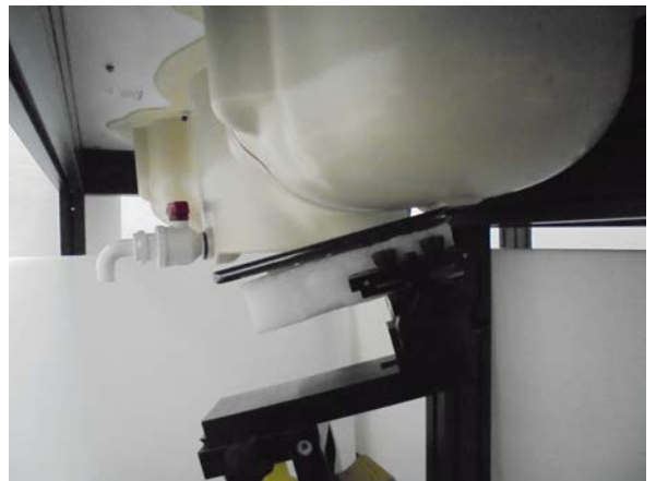
Figure 4. Left Head SAR Test Setup (Tilted)
