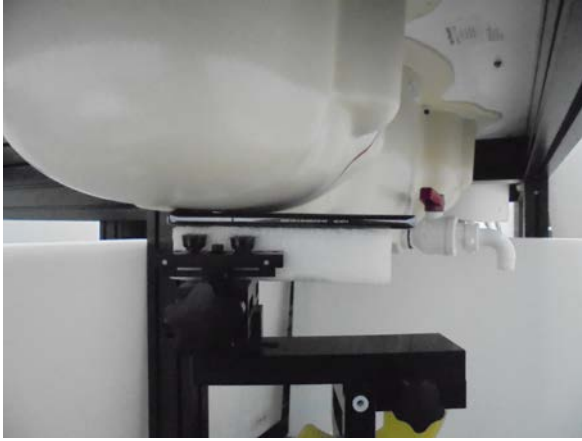
Figure 1. Right Head SAR Test Setup (Cheek)
