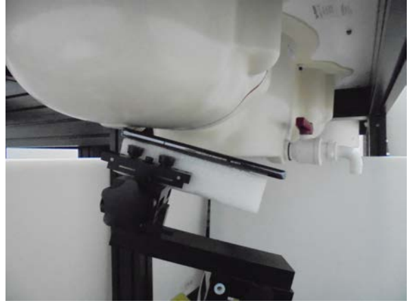
Figure 2. Right Head SAR Test Setup (Tilted)
