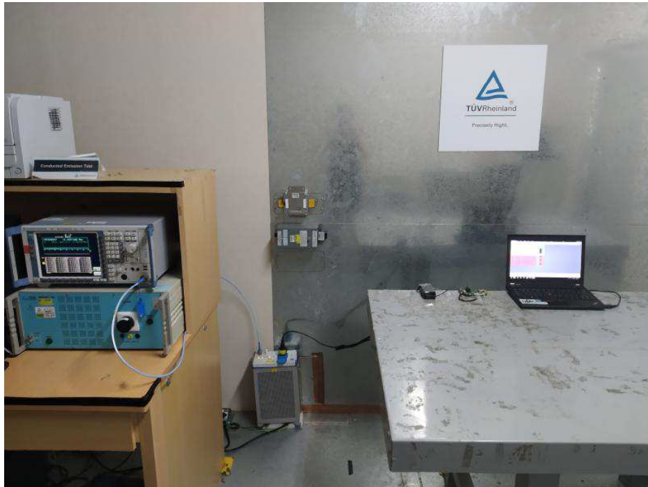
Photograph 19: Set-up for AC Mains (View 1)
