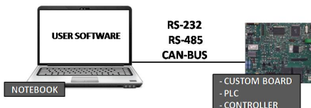
Figure B: example of local serial communication
