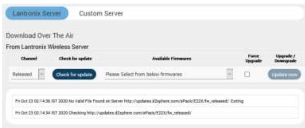
Figure 9.8-1. Download over the Air (DOTA) using Lantronix server
