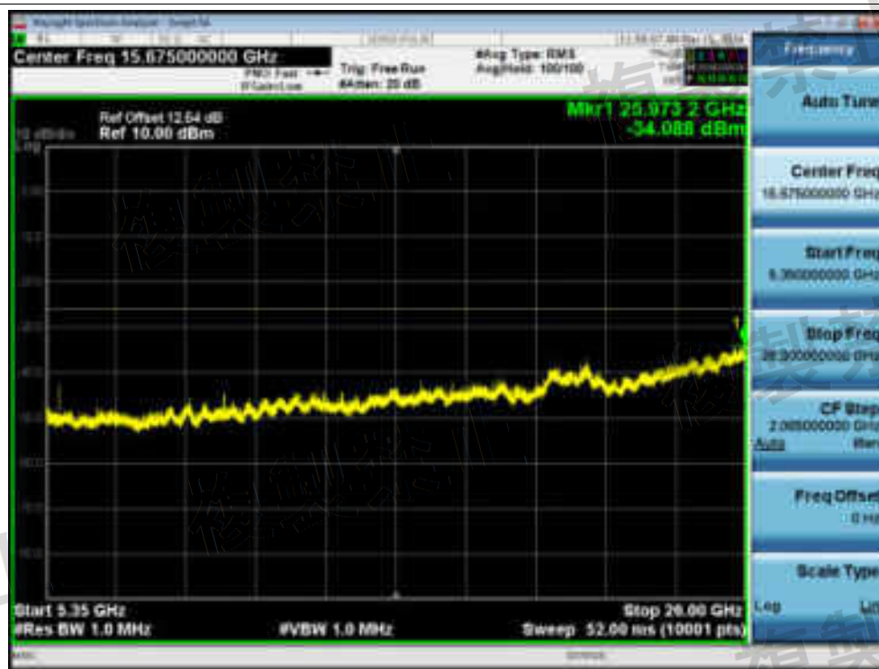
Tx. Spurious NVNT a 5300MHz Ant1 @ 5350MHz-26000MHz
