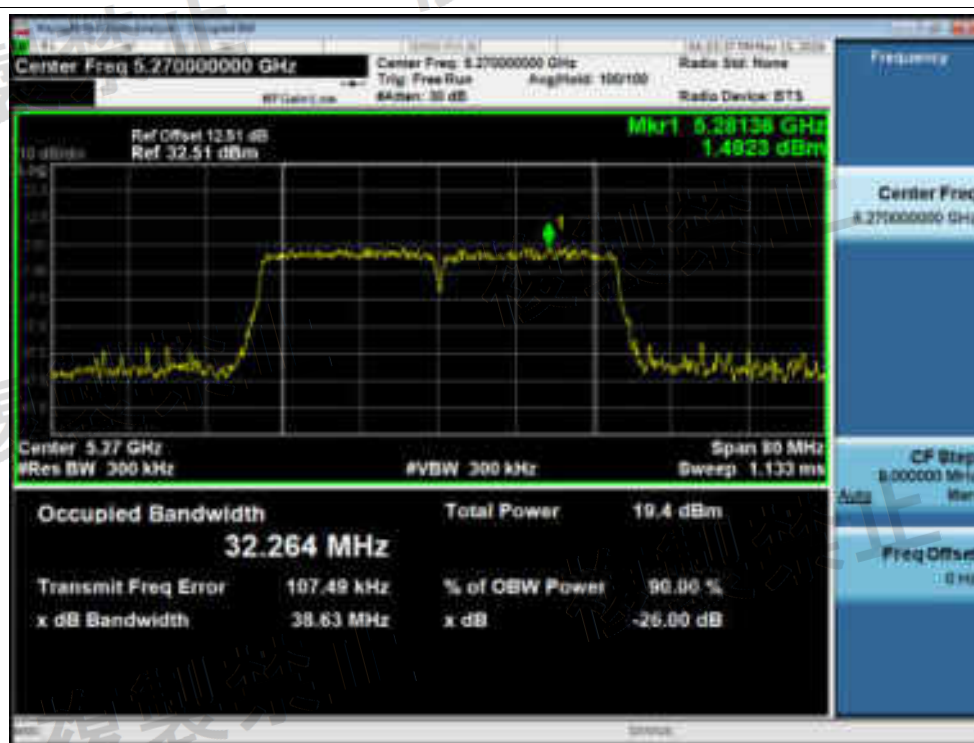
Spreading Bandwidth NVNT n40 5270MHz Ant1
