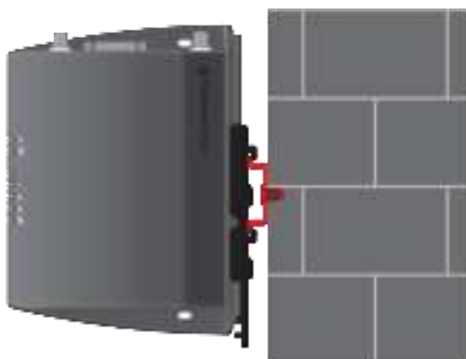
Figure 11 - Top hat DIN rail mount
