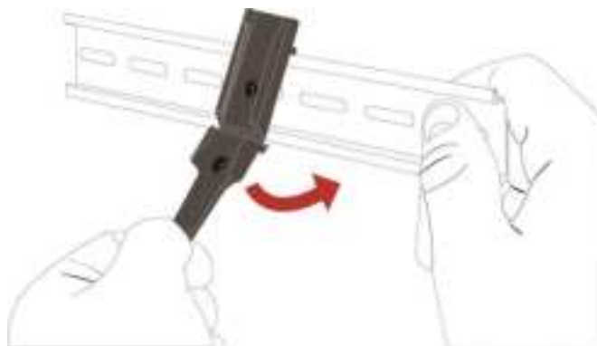
Figure 12 - Attaching the mounting bracket to the DIN rail using the V bend
