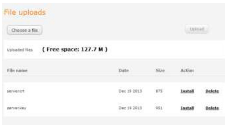
Figure 144 - Installing the server.crt file
