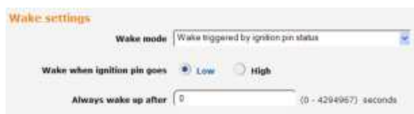
Figure 131 - Wake when triggered by ignition pin status
