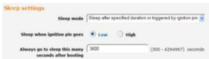
Figure 129 - Sleep after specified duration or triggered by ignition pin
