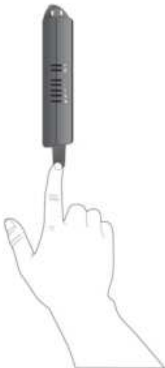
Figure 9 - Removing the mounting bracket
