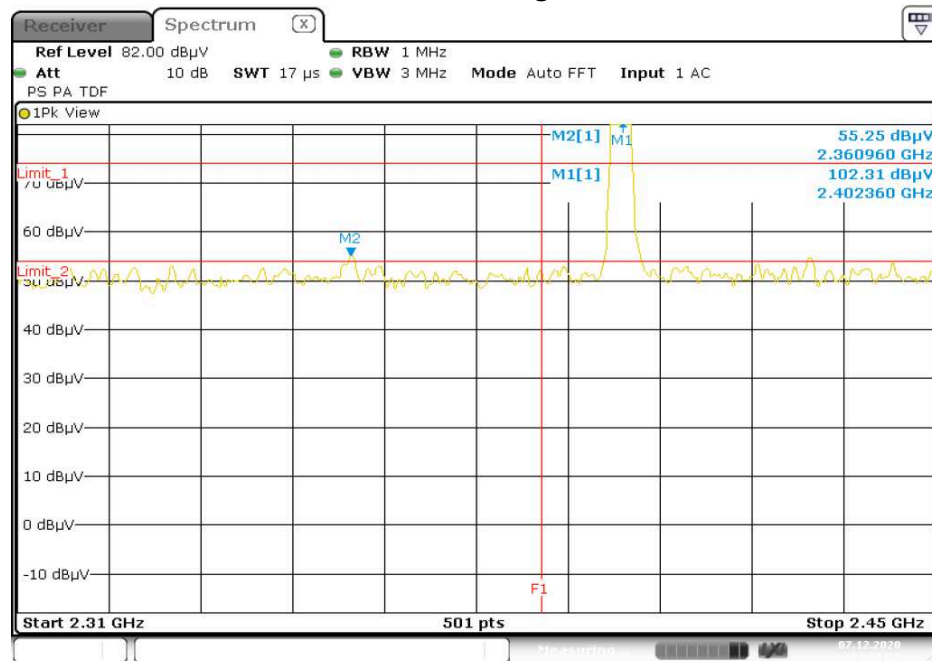
Chain0 : Restricted Band Bandedge @ BLE Mode Ch0 PK
