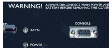
Figure 7. Internal RS-232 connector for the console
