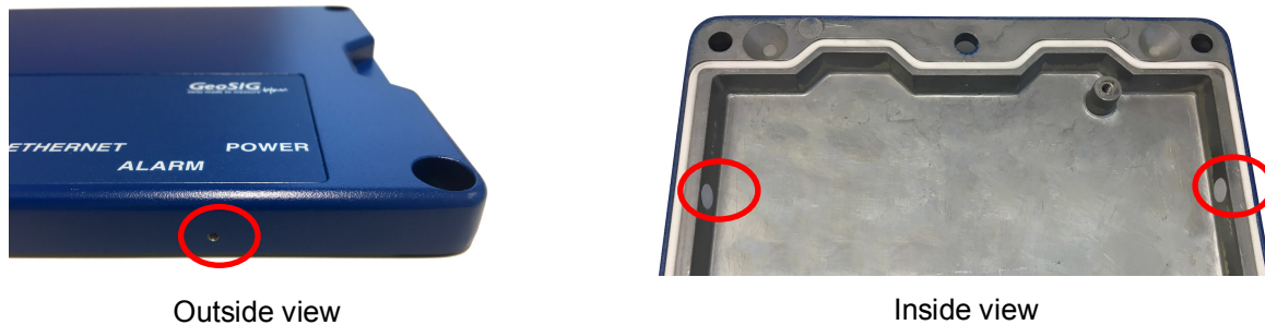
Figure 3. Housing lid ventilation holes
