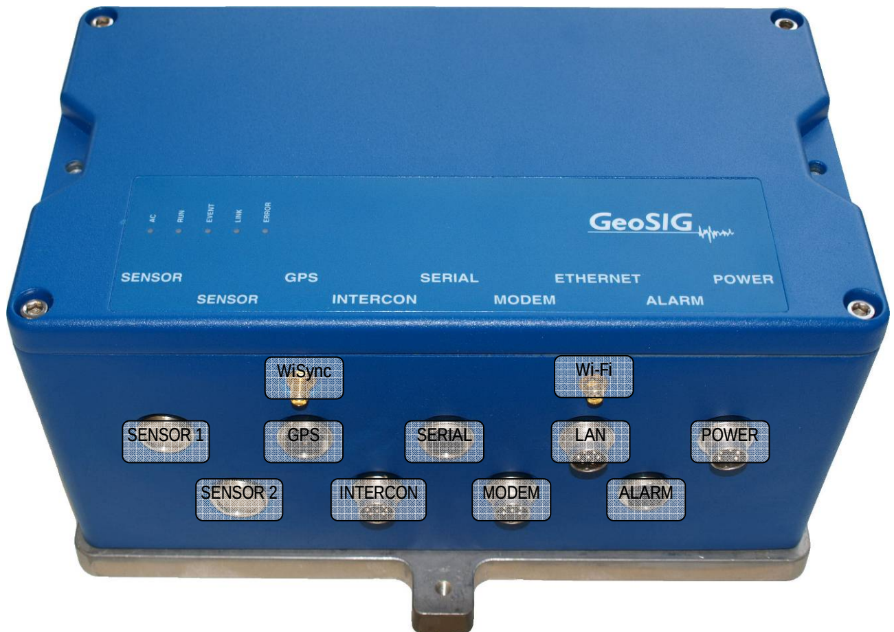
Figure 5. Instrument with all connectors. Antennas are not mounted. 2
