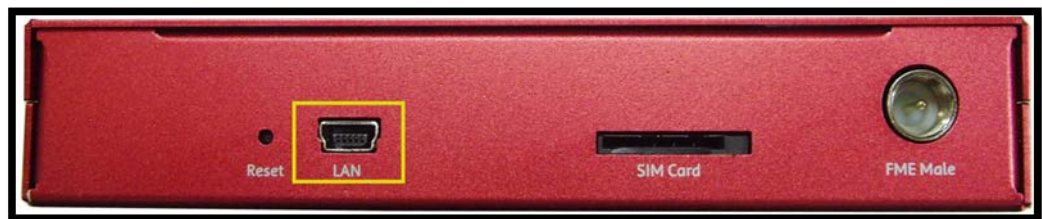
Figure1. Connect GPS module to LAN port
