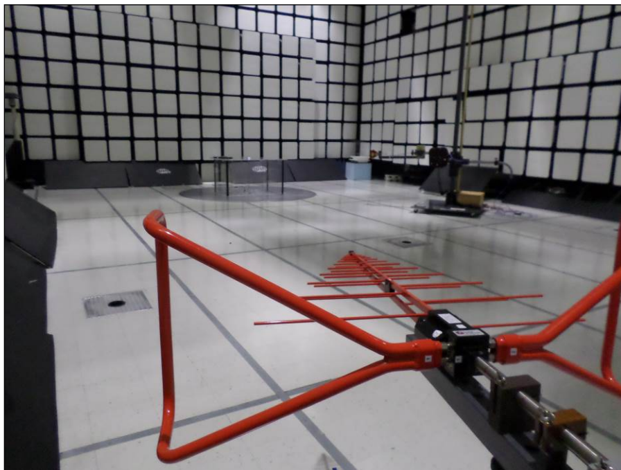
Photograph 4. Radiated Spurious Emissions, Test Setup, 30 MHz – 1 GHz, Antenna View
