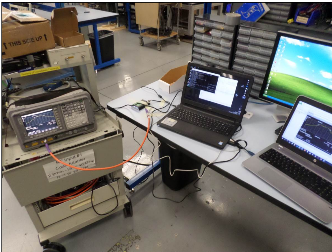
Photograph 3. Peak Output Power, Conducted Test Setup
