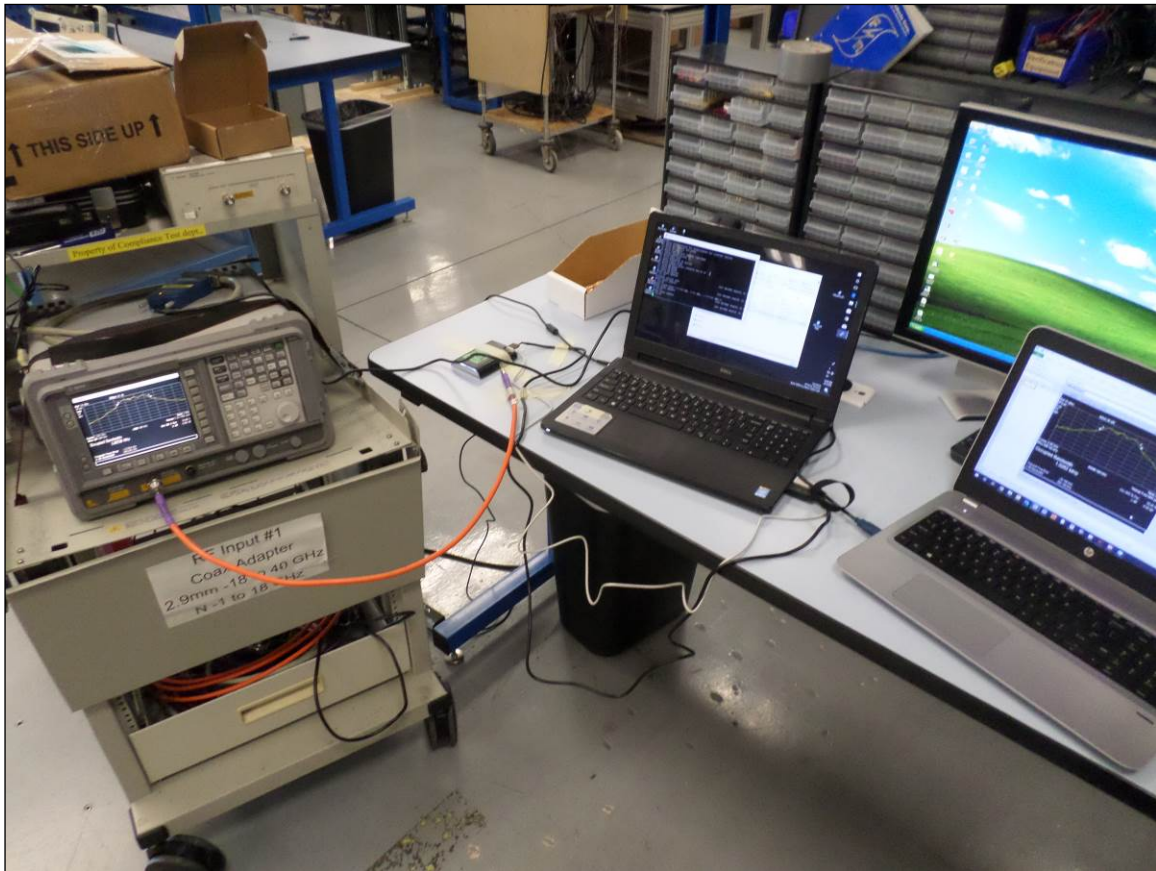
Photograph 12. Power Density, Conducted Test Setup
