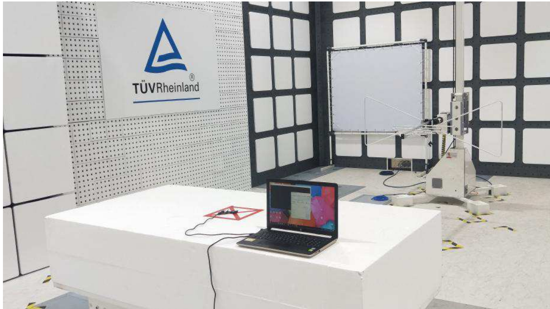
Photograph 5: Set-up for Spurious Emissions (Back View 3)
