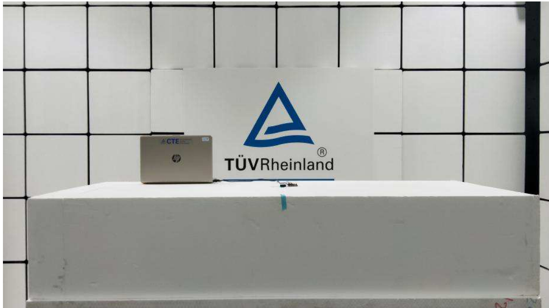
Photograph 1: Set-up for Spurious Emissions (Front View 1)
