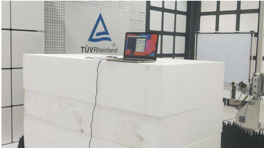
Photograph 3: Set-up for Spurious Emissions (Back View 1)
