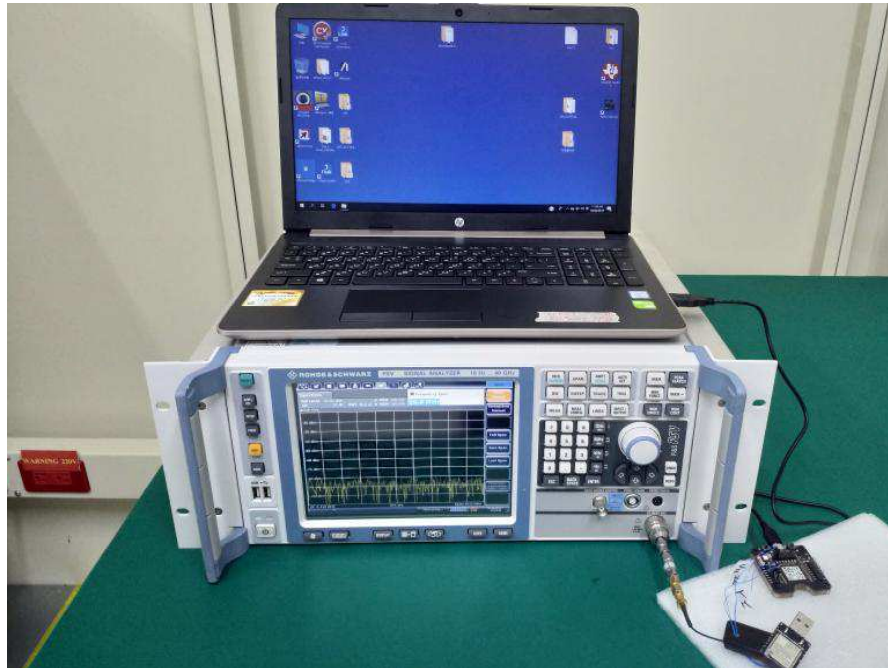
Photograph 7: Set-up for Conducted Test
