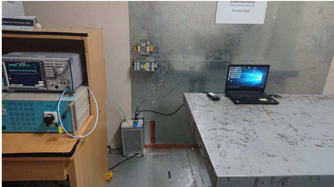
Photograph 9: Set-up for Mains Conducted Emissions
