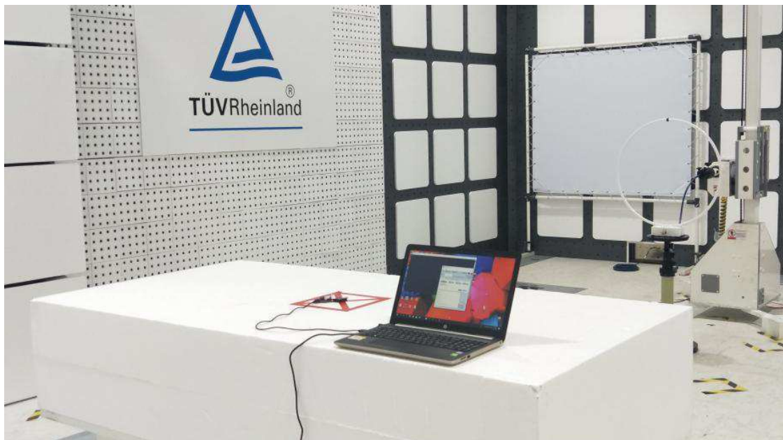
Photograph 6: Set-up for Spurious Emissions (Back View 4)
