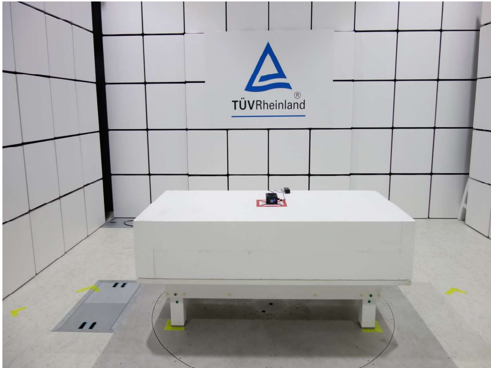
Photograph 1: Set-up for Spurious Emissions (Front View)
