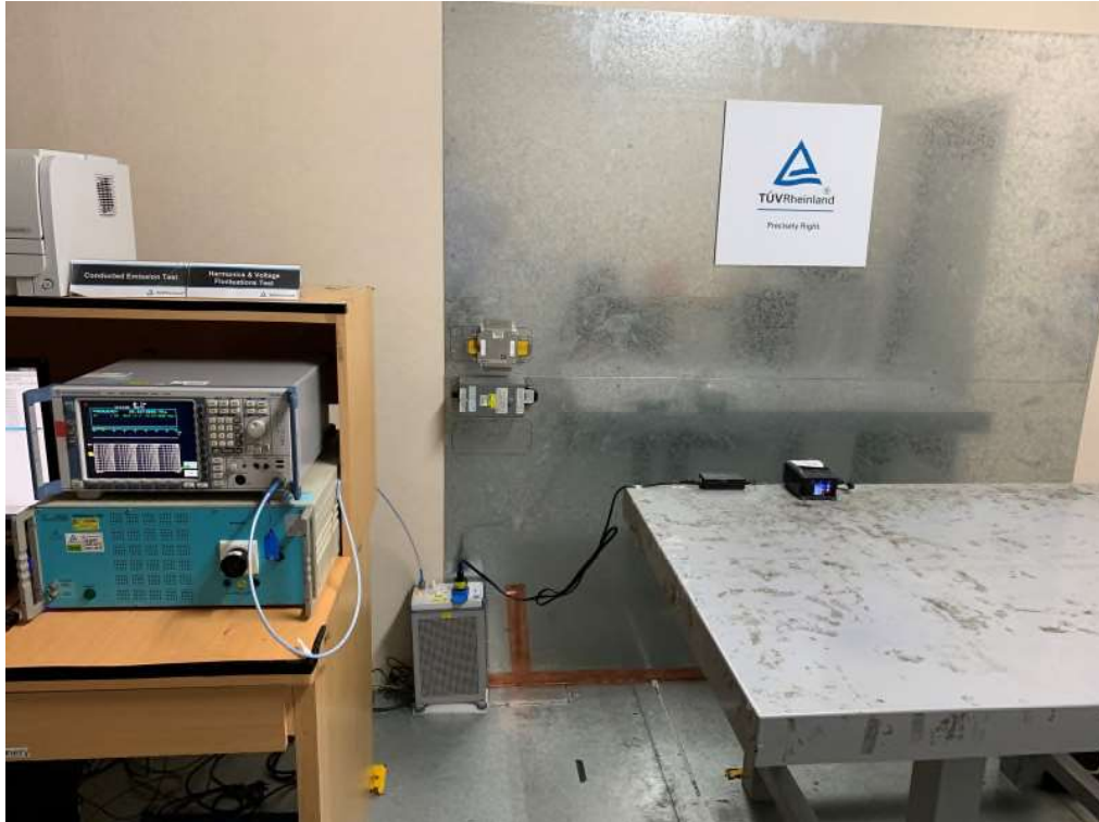
Photograph 5: Set-up for Mains Conducted testing (Front View)
