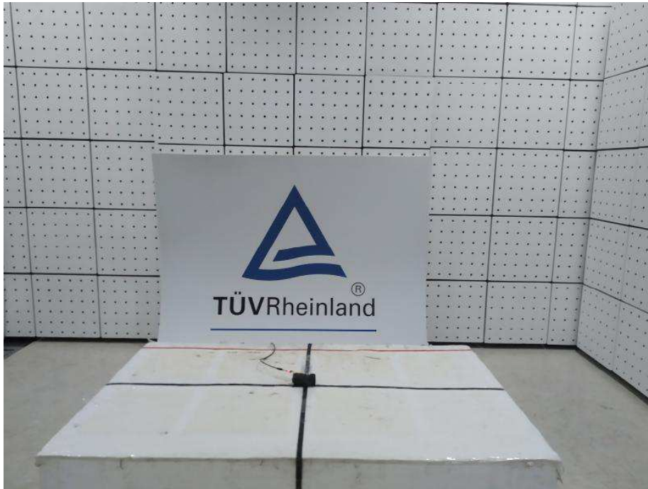
Photograph 2: Set-up for Spurious Emissions (Front View 2)
