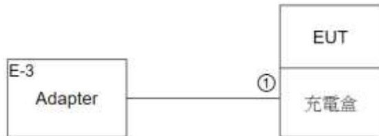
Conduction 量測配置圖(充電)
