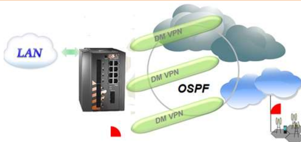
Figure 40 - L3 Protection Resilient Networking Between VPN Paths
