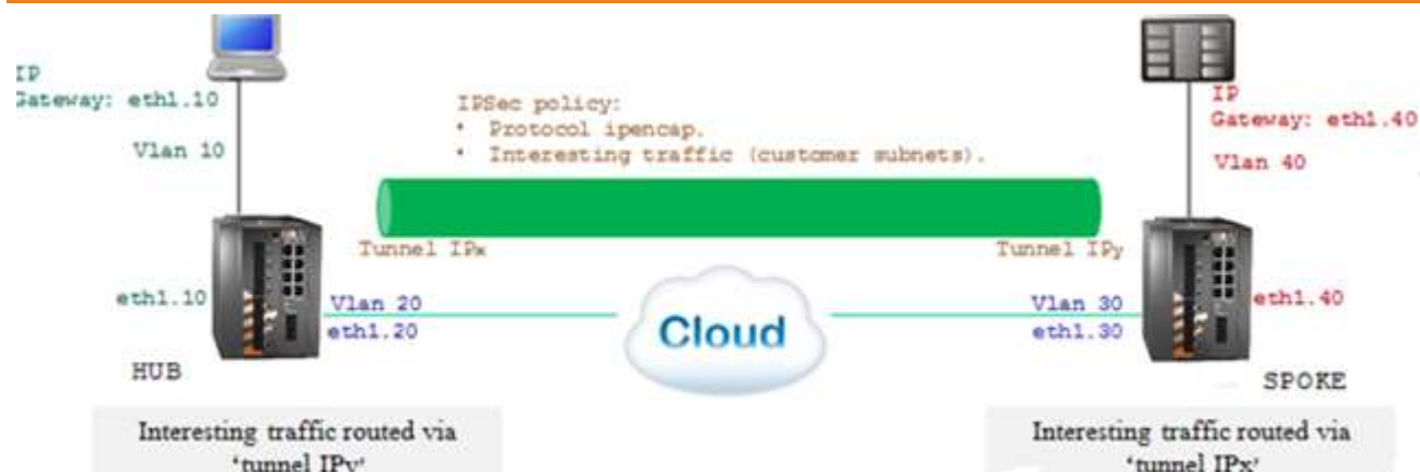
Figure 34 - Route Based IPsec-VPN
