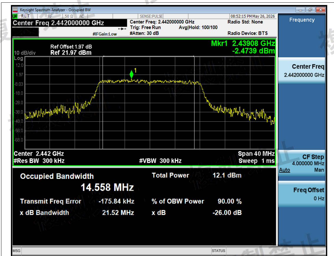
Spreading Bandwidth NVNT g 2442MHz Ant1
