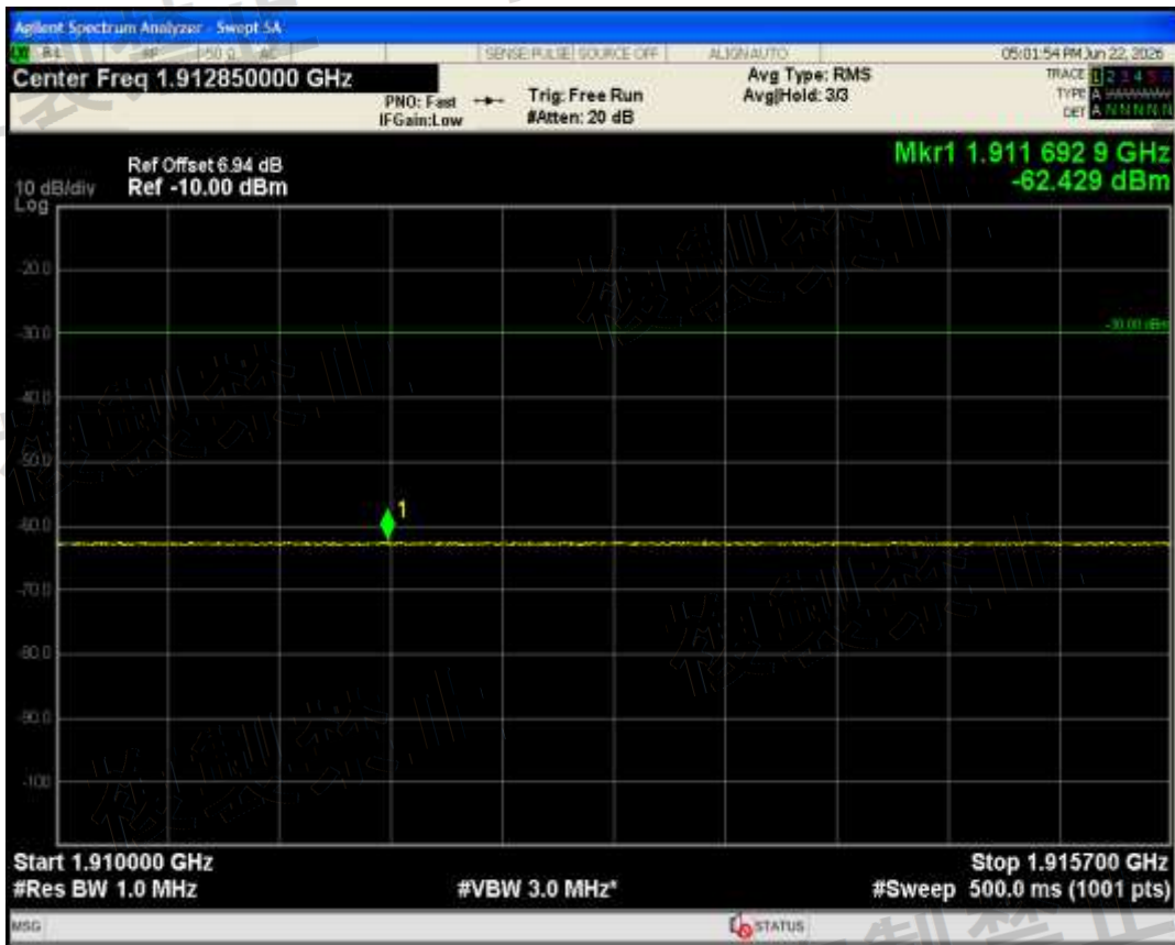
Band3(1750-1785) QPSK BW=5MHz Channel=19625 RB Size=1 Position=#Max Range2010 MHz-2025 MHz
