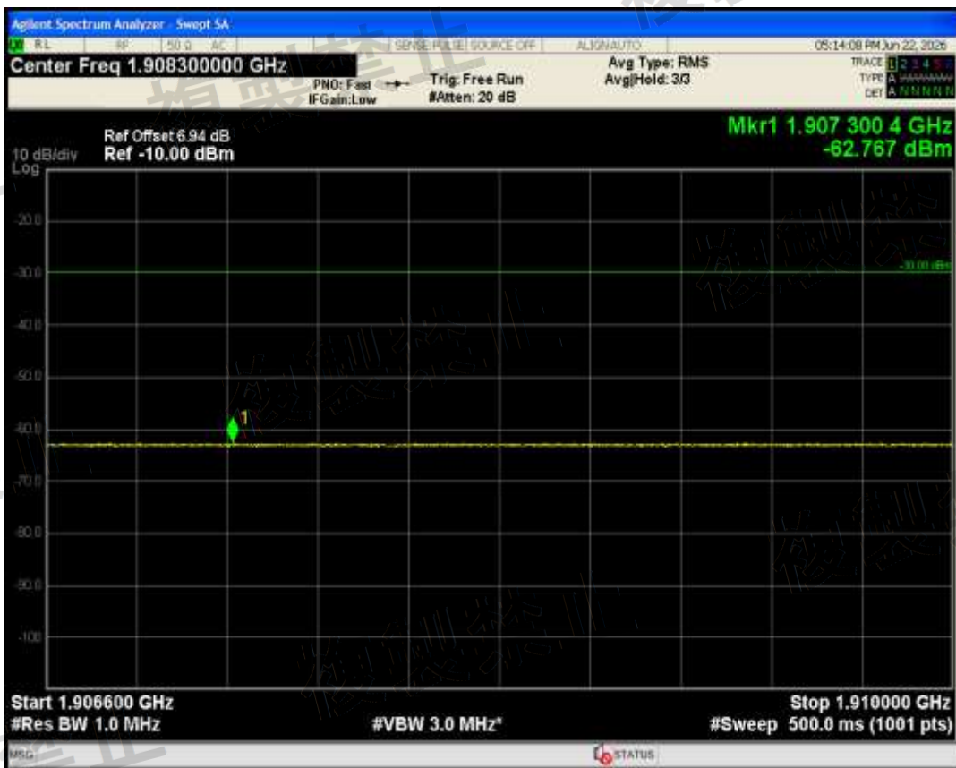
Band3(1750-1785) QPSK BW=5MHz Channel=19775 RB Size=25 Position=#0 Range1910 MHz-1915.7 MHz
