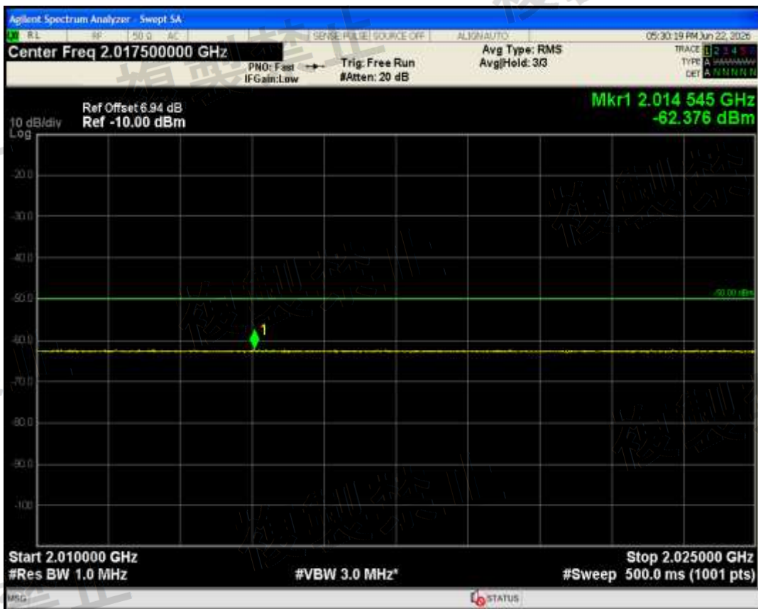
Band3(1750-1785) QAM16 BW=5MHz Channel=19925 RB Size=25 Position=#0 Range2144.4 MHz-2170 MHz
