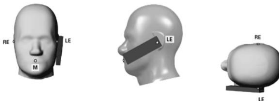
Fig 11.2.3 cheek or touch position. The reference points for the right ear (RE), left ear (LE), and mouth (M), which establish the Reference Plane for handset positioning, are indicated.
