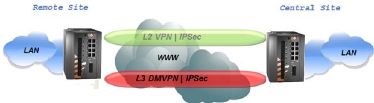
Figure 31 - IPsec Encrypted Link Topology
