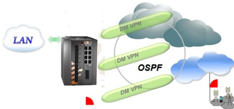
Figure 40 - L3 Protection Resilient Networking Between VPN Paths
