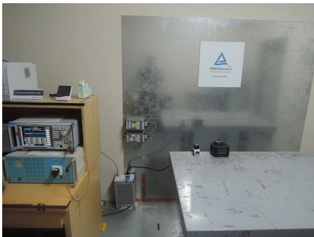
Photograph 4: Set-up for Spurious Emissions, AC Mains (Front View)
