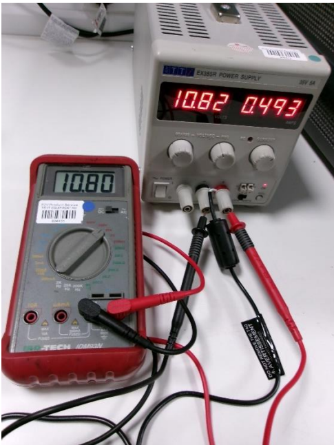
Figure 1 - Photograph showing V(in) setup for the minimum DC voltage (10.8V).
