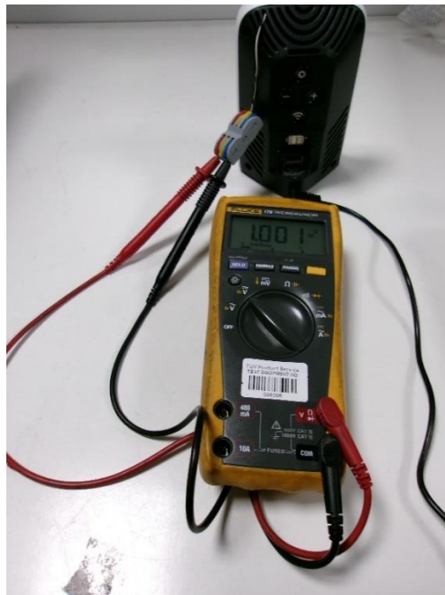
Figure 4 : Photograph showing the voltage was measured to the RF Circuitry socket (V(in) = 12.0 V DC at DC socket input)
