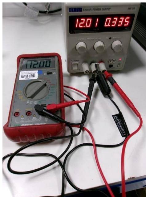
Figure 3 - Photograph showing V(\text{in}) setup for the nominal DC voltage (12.0V).
