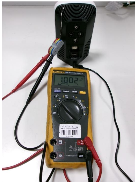
Figure 2 - Photograph showing the voltage was measured to the RF Circuitry socket ( V_{\min} = 10.8 \text{ V DC} at DC socket input)
