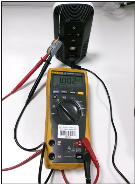
Figure 6 - Photograph showing the test point at which the voltage was measured to the RF Circuitry (V_in = 13.2V DC at DC input socket)
