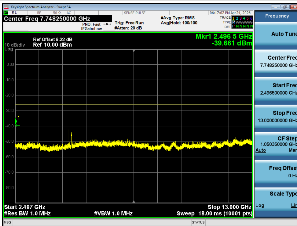
Tx. Spurious NVNT 2-DH5 2441MHz Ant1 @ 2496.5MHz-13000MHz
