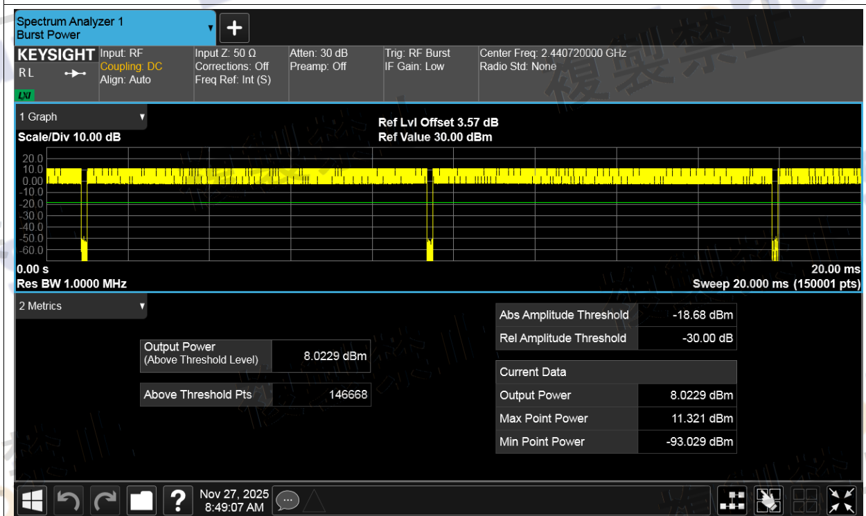
Power NVNT b 2472MHz Ant1 Pre Scan
