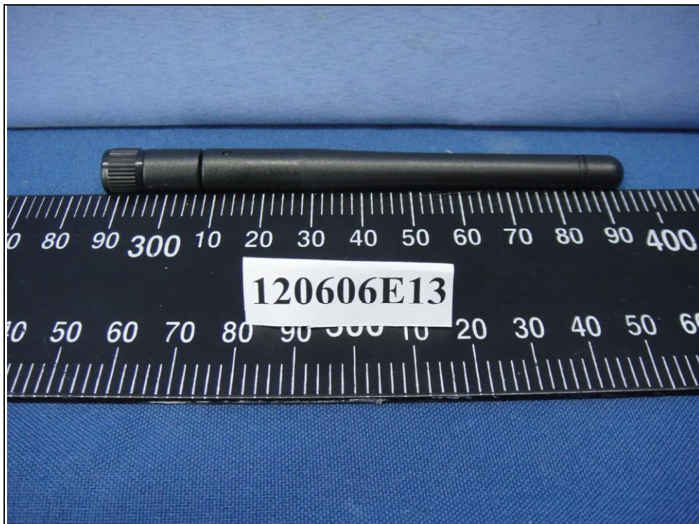
Antenna set 5 Dipole Antenna (Brand name: WHA YU GROUP, Model No.: C1336S510077-A)
