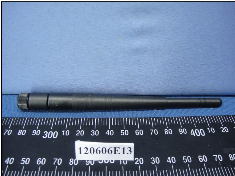
Antenna set 6 Dipole Antenna (Brand name: WHA YU GROUP, Model No.: C529-510331-A)
