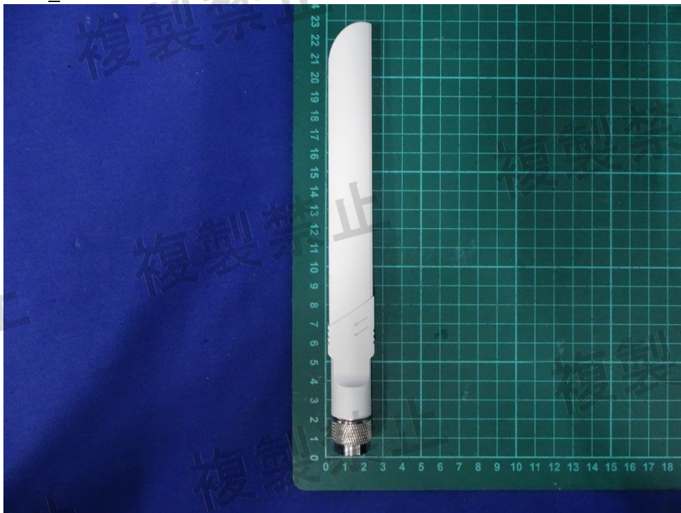
(40) EUT Photo_ Antenna: MOXA / ANT-WDB-ANM-0306
