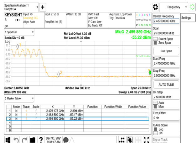
Hopping Band Edge_GFSK_1M_DH5_2480MHz
