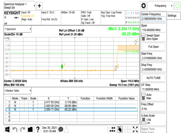
Hopping Band Edge_GFSK_1M_DH5_2480MHz
