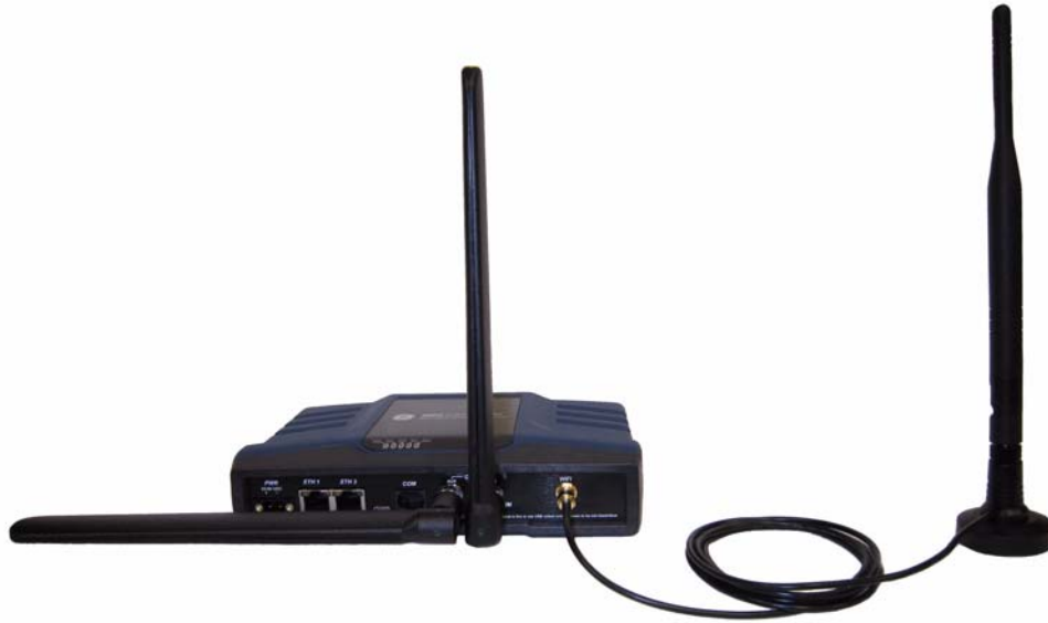
Figure 10. Direct Mounting of Cell Antenna; Cabled WiFi Antenna Minimum 8-inch (20.32 cm) separation between cell and WiFi antennas
