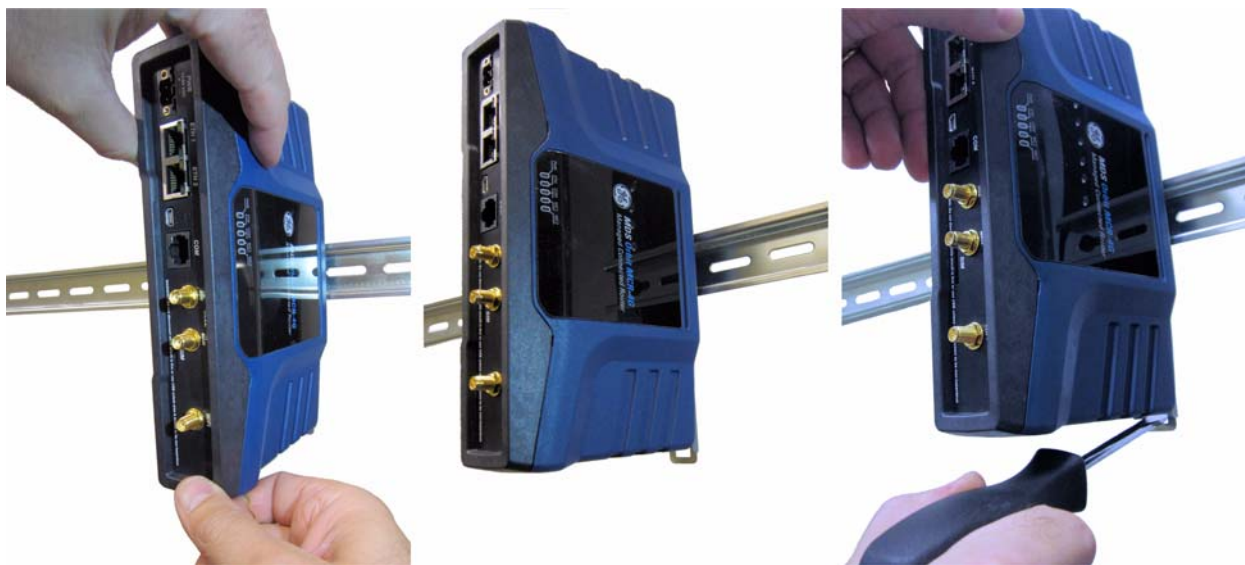
Figure 9. DIN Rail Attachment and Removal (Pull down tab to release from rail)
