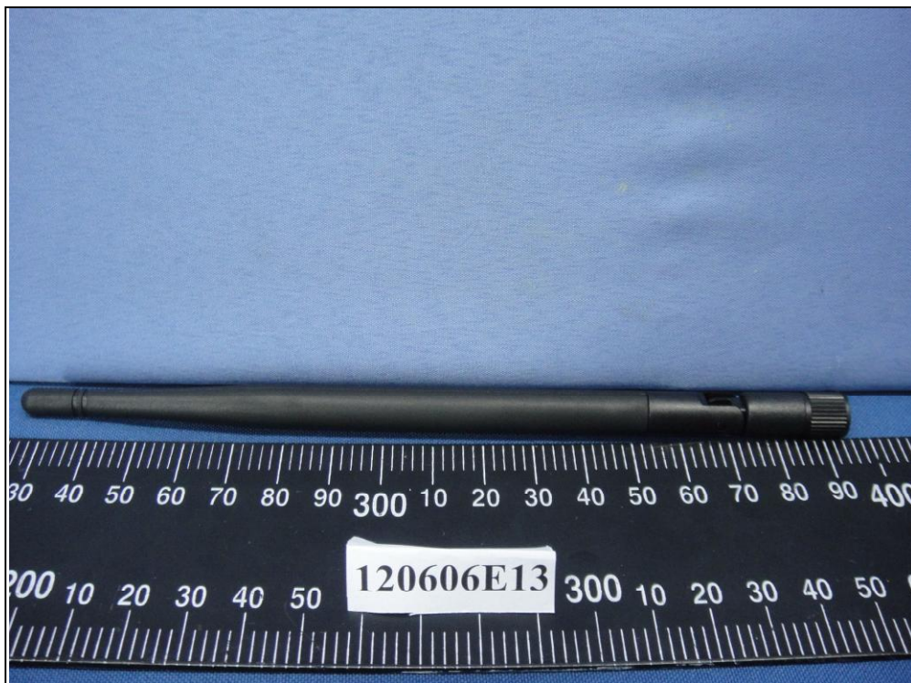
Antenna set 9 Dipole Antenna (Brand name: WANSHIH ELECTRONIC CO., LTD, Model No.: WSS007)
