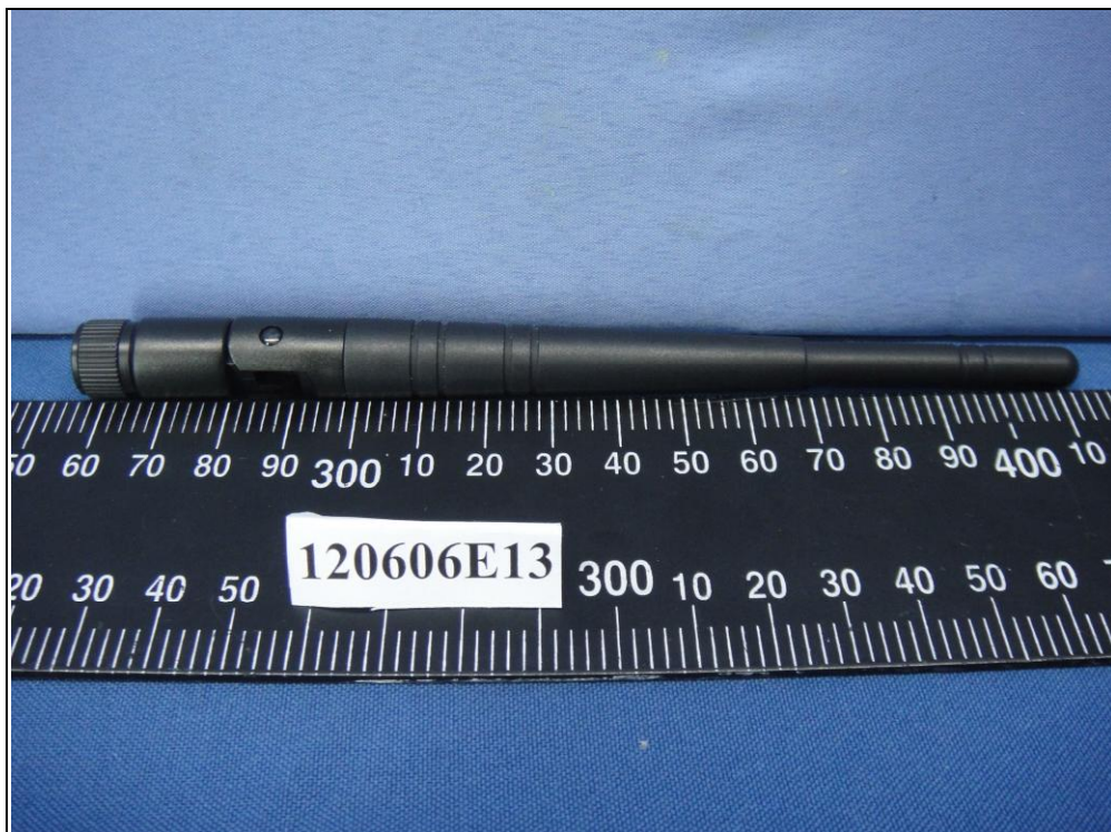
Antenna set 8 Dipole Antenna (Brand name: WANSHIH ELECTRONIC CO., LTD, Model No.: WSS003)
