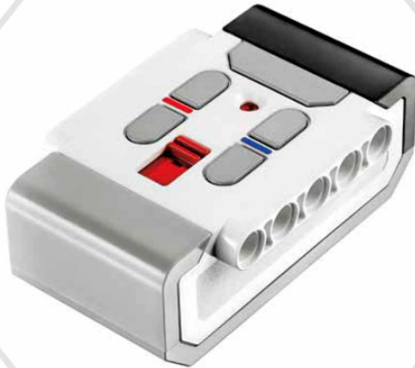
Remote Infrared Beacon
