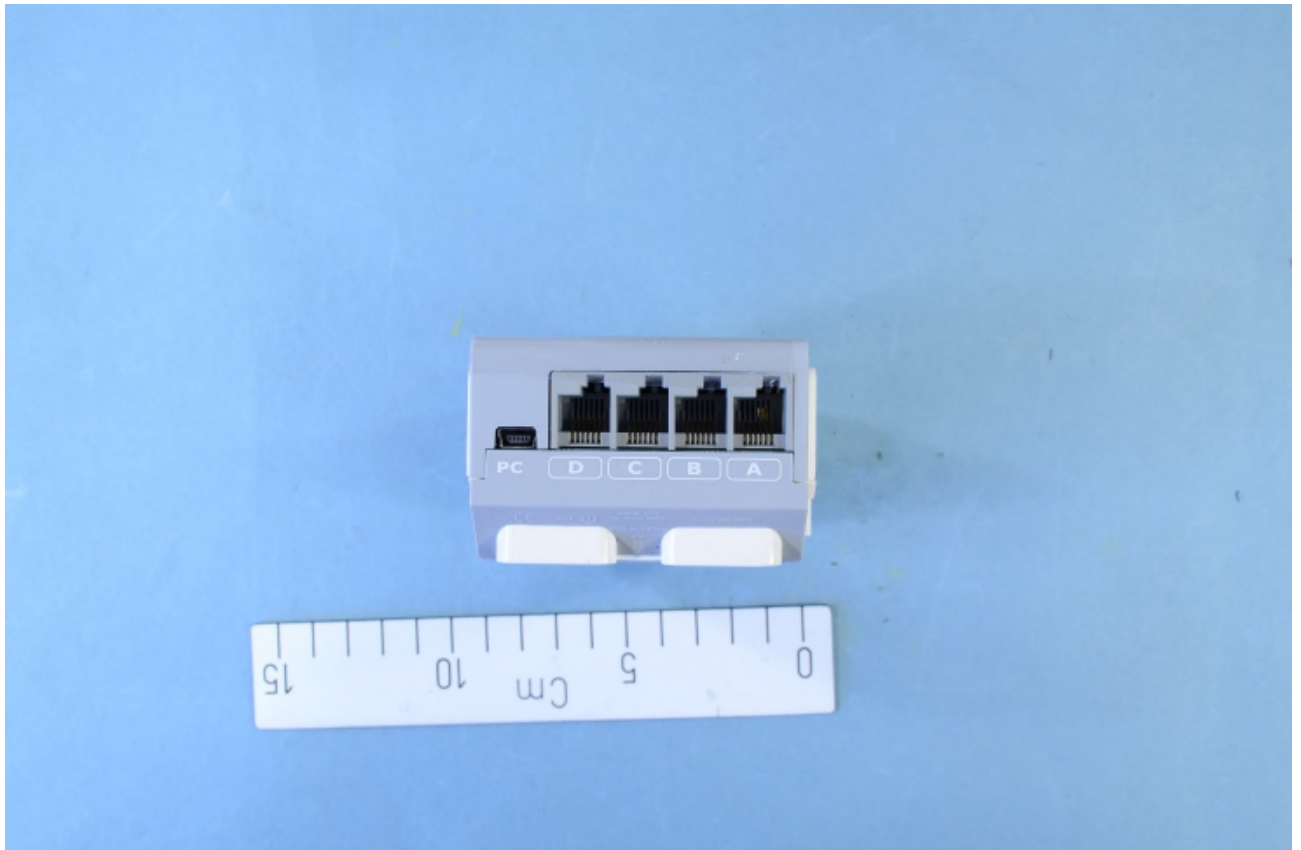
Side view 1 (motor & sensor ports view)
