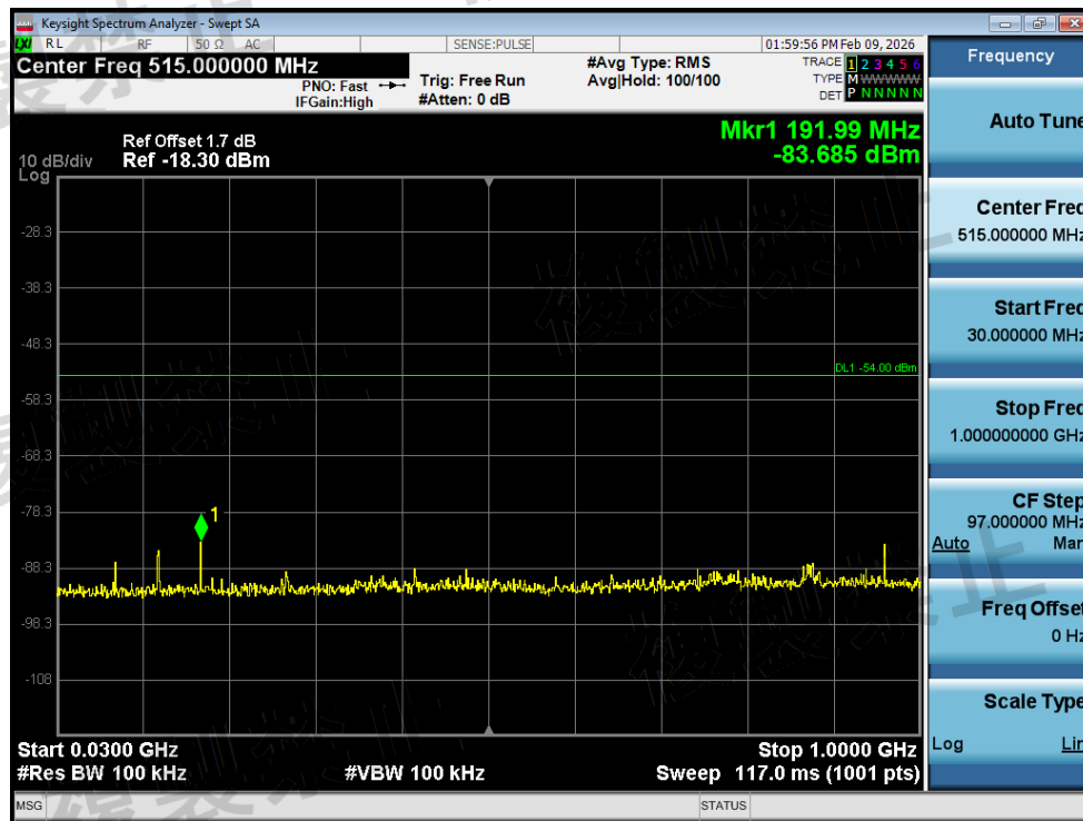
Rx. Spurious NVNT GFSK 2430MHz Ant1 @ 30MHz-1000MHz
