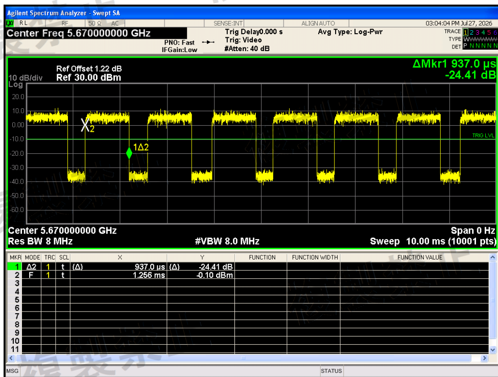
Burst Length NVNT ax20 5500MHz Ant1
