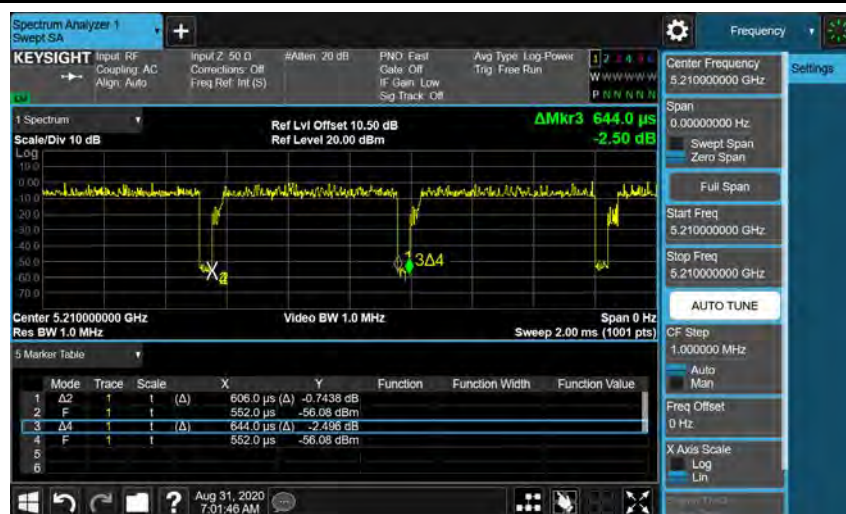
Mode 11: IEEE 802.11ac 80 MHz Continuous TX Mode
