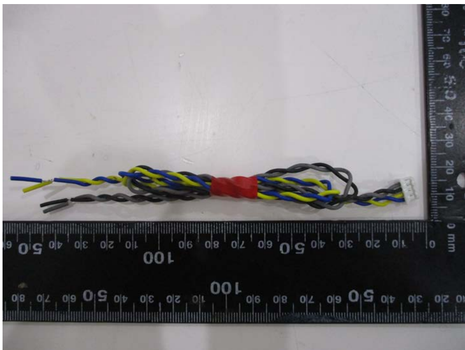
connection cable 4 pins(RS-485)
