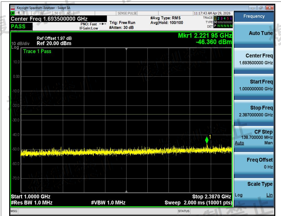
Tx. Spurious NVNT BLE 1M 2440MHz Ant1 @ 1000MHz-2387MHz
