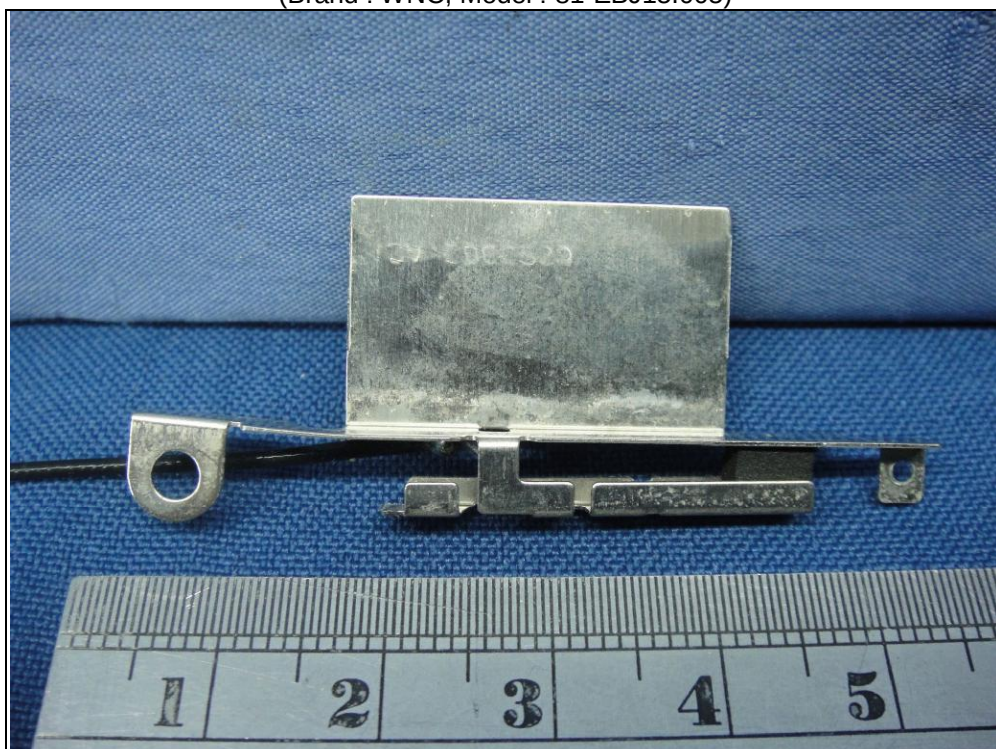
Antenna set 1 – No.1 (Brand : WNC, Model : 81-EBJ15.005)
