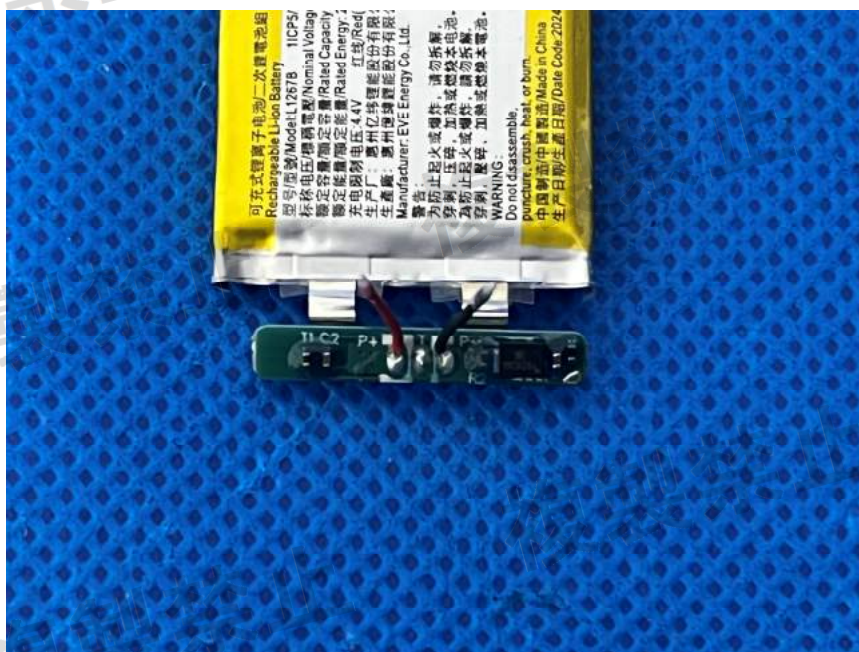
Figure 18: Protective board of charging case battery
