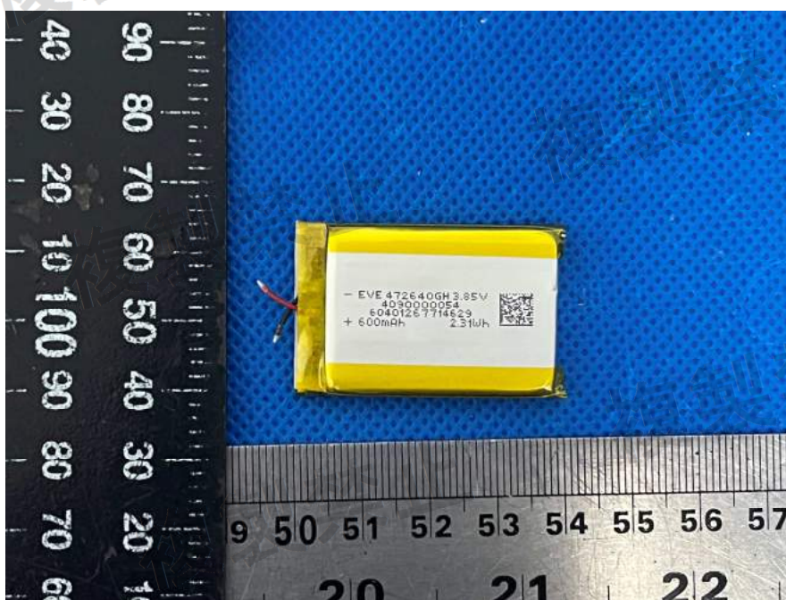
Figure 17: Battery view of charging case
