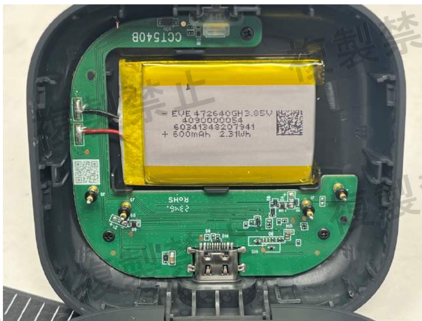
Figure 8: Internal view of charging case
